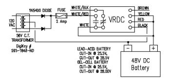
The emergency battery needs to be charged in a reasonable time after use. The VRDC 24V-60 senses the battery voltage, starts the charging current when the voltage drops below a threshold and disconnects the charging current when the battery is fully charged.
