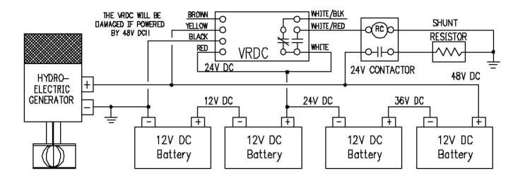
The VRDC 24V-60 senses the battery voltage and activates a contactor to shunt the excessive power thru a load resistor to prevent an over voltage condition. The VRDC 24V must be powered by 12 DC from the battery bank even though it senses a higher voltage level thru the series input resistor.
