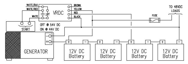
The VRDC 24V/60 senses when the battery bank is being discharged below a threshold point and starts the generator to charge the batteries. It shuts off the generator when the desired battery voltage is achieved. The time delay prevents the generator from starting on temporary battery voltage drops.
