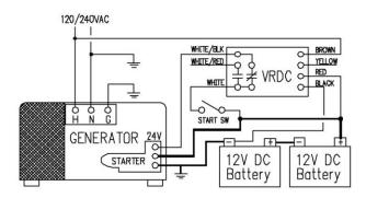
The VRDC 24V-60 senses the AC voltage output from a generator and when the desired threshold is reached, disconnects the starter circuit to prevent excessive cranking. Even though the AC voltage adjustment is 150VAC maximum, the module is not damaged by seeing 240VAC on the voltage input wire.
