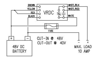
The VRDC 24V-60 energizes and disconnects the load (with time delay) below the off voltage point to prevent further battery discharge. Use N.O. contacts for de-energize on low battery voltage condition.
