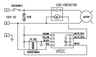
The VRDC 24V-60 senses the AC line voltage and disconnects a motor or other sensitive load if the low voltage condition persists past the time delay period. The time delay prevents the VRDC from dropping out the motor due to normal inrush current draw. Cut out below 105VAC, cut in @ 112VAC.
