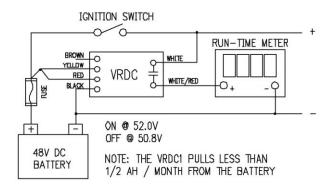
The VRDC 24V-60 senses the alternator output and energizes the run-time meter only when the engine is running and the ignition is on. This prevents the meter from running needlessly when the ignition is left on as is often the case with recreational boats.
