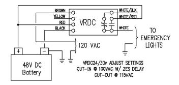
The VRDC 24V-60 senses the 120VAC line voltage and switches on the emergency lights with a 2 second delay upon sensing a power failure. The emergency lights turn off when power returns.
